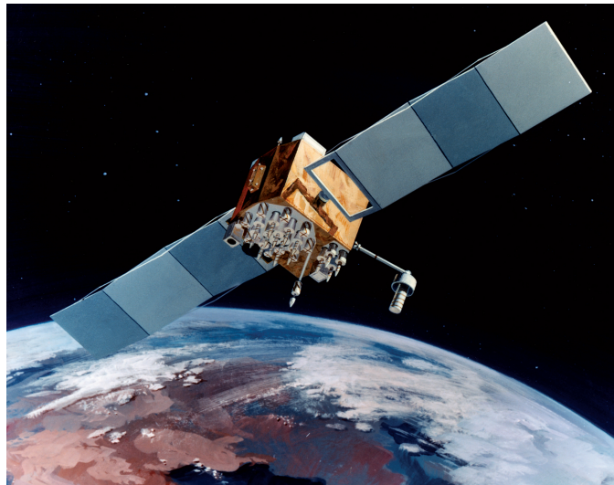
Figure 1: Navstar-2F satellite of the Global Positioning System. Figure source, USAF, released into the public domain. https://en.wikipedia.org/wiki/GPS_Block_IIF#/media/File:Navstar-2F.jpg .
